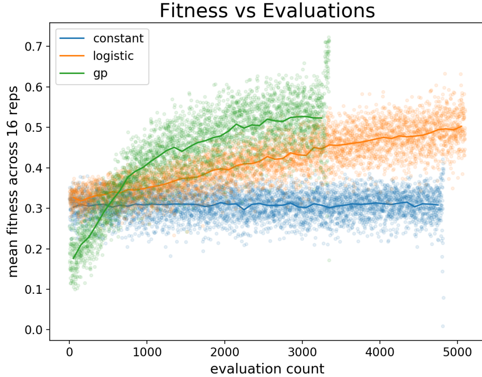
Figure 3.4: The GP model shows an initial fitness of 0.19, lower than both the constant and Logistic model. Both alternative models have implicitly bounded output while the GP must learn the correct domain over time.
