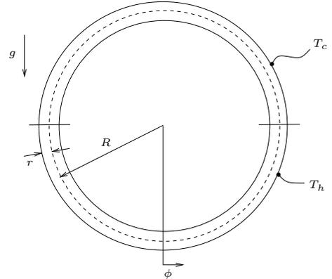
Fig. 1: The thermosyphon has a simple toroidal geometry. The bottom wall is heated to a constant hot temperature  $T_h$  while the top wall is maintained at the temperature  $T_c$ . This creates a temperature inversion of hot fluid below cold, an unstable situation. Energy in the bottom half must find a way to the top half. If conduction alone cannot stabilize this temperature inversion, then the fluid will start to move and convection becomes the dominant method of heat transfer.
