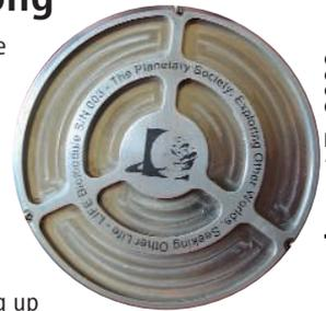
The Living Interplanetary Flight Experiment (LIFE), designed and sponsored by the Planetary Society in Pasadena, California, will hitch a ride on a Russian sample-return mission to Mars's moon Phobos to see whether Earth life without special protection can survive a 34-month space voyage. "We view this as a simulated meteoroid," says Bruce Betts, the society's director of projects.
