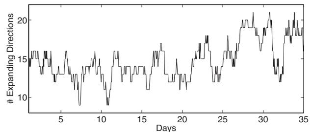
FIG. 3. In the 40 dimensional system discussed later, the number of expanding directions varies from 8 to 23 depending on the state investigated. As a trajectory is followed, the same fluctuations in the local number of expanding directions are observed.
