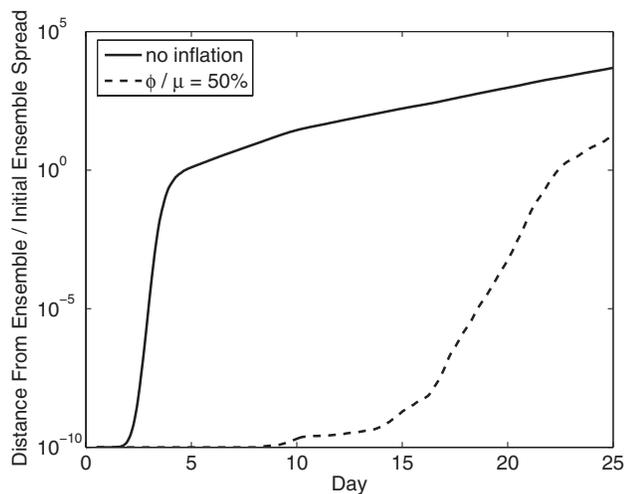
FIG. 5. The distance between an  $H$  trajectory and the nearest trajectory of the ensemble ellipsoid is plotted vs time, averaged over 5000 independent 25-day ensemble forecasts (solid) and their corresponding continually inflated ensemble forecasts (dotted). The vertical axis is in units of the initial diameter of the ensemble.
